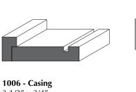
1006 - Casing 3 1/2" x 3/4" 1205 - Backband 1 1/4" x 3/4" with 3/4" rebate
